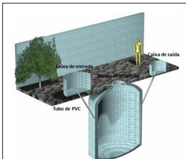
FIGURA 2: BIODIGESTOR CHINÊS.
