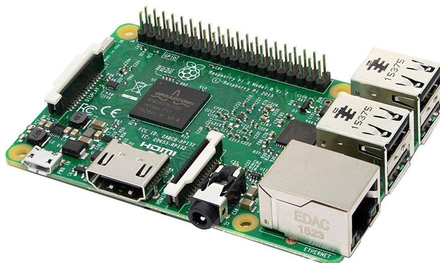
Figura 13 - Raspberry PI 3 Model B
